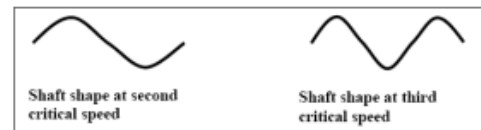
Figure 4. Typical shaft shapes at second and third critical speeds.
