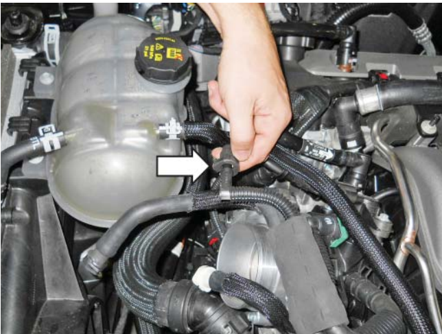
25. Disconnect the throttle body electrical connector. Pull the red locking tab back; press the black release tab to disengage the lock.
