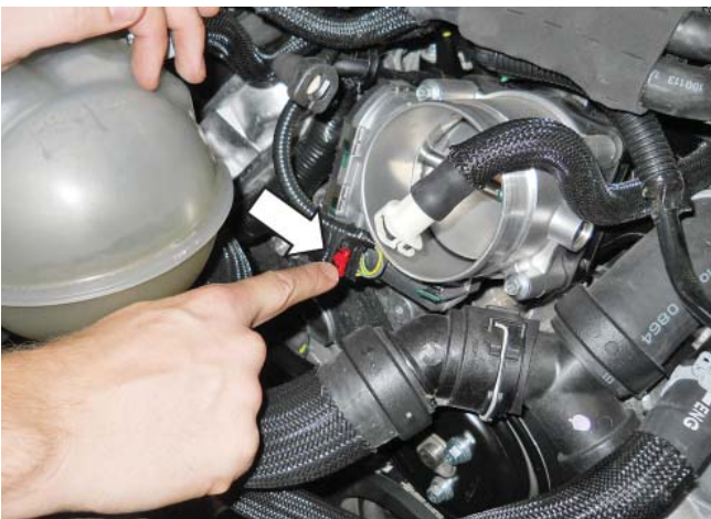
25. Disconnect the throttle body electrical connector. Pull the red locking tab back; press the black release tab to disengage the lock.
