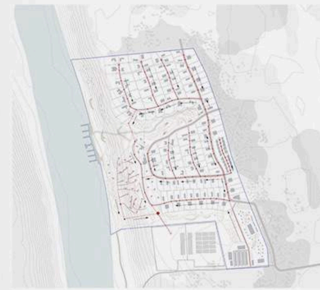
Master Plan with a Water Sewer Scheme
